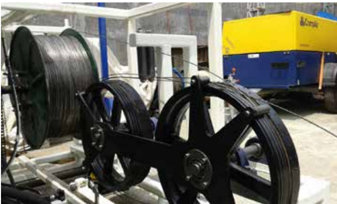
Capstan with the band brakes.
