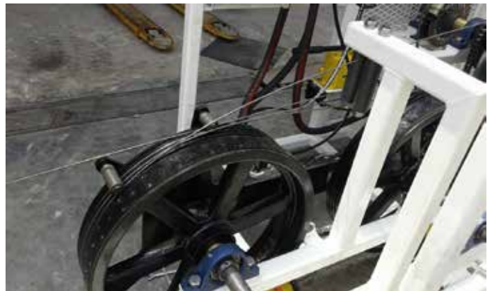
Capstan with the band brakes.
